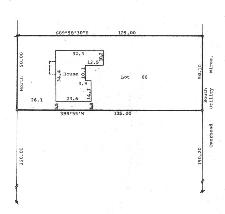
Scale -1" = 20"●= 1" Dia. Iron Pipe Found →= 3/4" Dia. Iron Pipe Found ♦= ½" Dia. Iron Pipe Found 0 = 3/4"x24" Iron Pipe Set (0.00) = Recorded Distance
